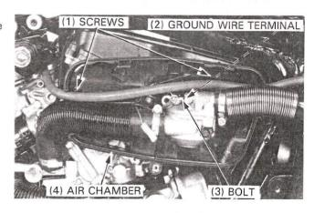
Remove the left air chamber and screws. Remove the No. 2 spark plug cap.
