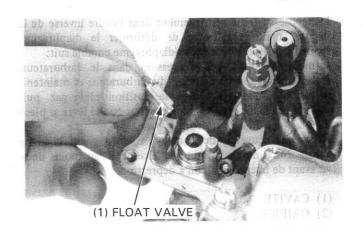
Remove the starter jet, main jet and slow jet. Remove the float valve seat and filter. Remove the needle jet holder and needle jet.
