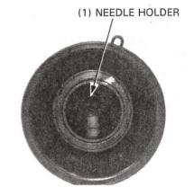
Inspect the needle for excessive wear at the tip and for bending or other damage.
