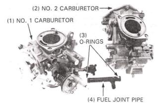
Reconnect the throttle linkage between the No. 1 and No. 2 carburetors using new cotter pins.
