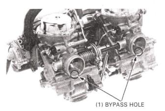
Align each throttle valve with the bypass hole edge by turning the synchronization adjusting screws.
