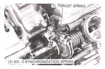
Install the synchronization springs between the No. 2 and No. 4 carburetor throttle arm, throttle link arm and the thrust springs between the throttle shafts.
