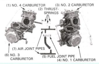
Remove the choke rod cotter pins and choke rod from the No. 1 and No. 2 carburetors.
