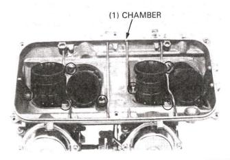
Carefully separate the No. 1 and No. 2 carburetors from the No. 3 and No. 4 carburetors.
