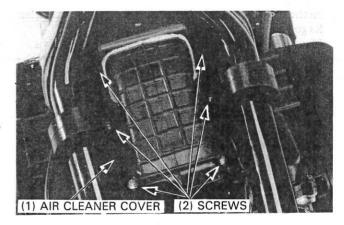
Disconnect the breather tube from the air cleaner. Remove the following:
