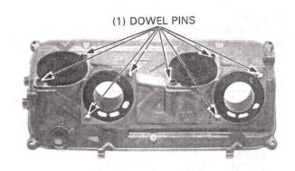
Place the air chamber over the carburetors, aligning the dowel pins with the carburetor holes.
