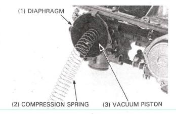
Push the needle holder in and turn it 60 degrees with an 8 mm socket. Then remove the needle holder, spring and needle from the piston.
