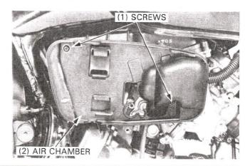
Remove the air cleaner case (page 4-13). Disconnect the breather hose from the air cleaner case.
