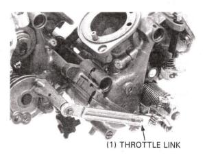
Remove the screw from the No. 1 carburetor. Carefully separate the No. 1 and No. 2 carburetors.
