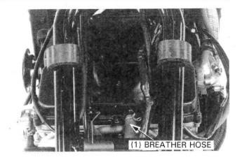
Disconnect the automatic fuel valve tube from the intake manifold.
